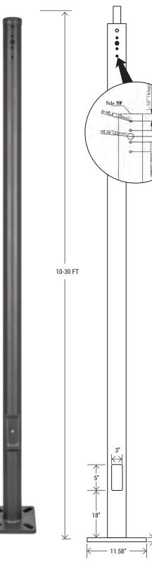
The JMC Series Straight Round Steel poles are built from high strength steel tube and are available side drilled for arm mounted area lighting luminaires or with tenon mounts for flood and post top luminaires. Typical area lighting applications include retail centers, industrial parks, schools and universities, public transit and airports, office buildings and medical facilities. Mounting heights of 10 to 30 feet can be used based on selected luminaire application.
